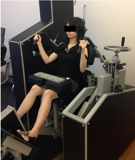
Fig. 1. A participant is seated on MedX Lumbar Dynamometer at 12° lumbar flexion. Full extension is defined as 0° lumbar flexion and full flexion is 72° lumbar flexion.
